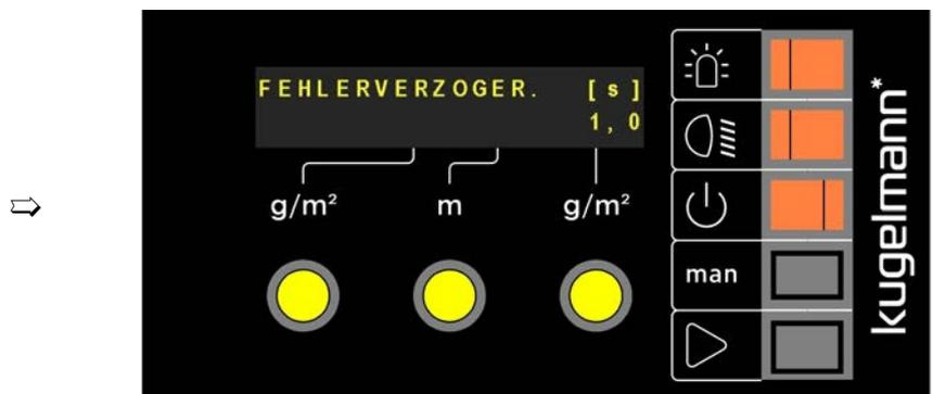
3 Set desired error delay time at the right-hand turning knob (0.0 , ..., 60.0 s).
