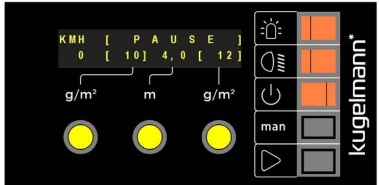
Example for basic setting of spreading width (4.0 m).
