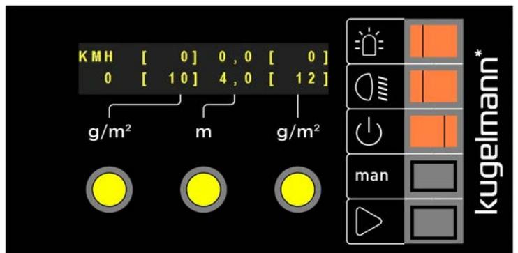
Spreading starts as soon as the carrier vehicle starts to move.
