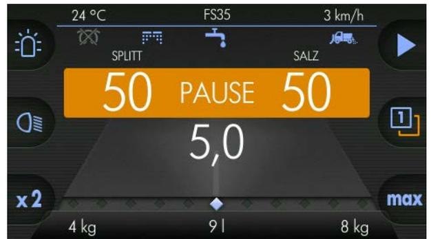
Turn middle turning knob to set spreading width (4,5 m) →
