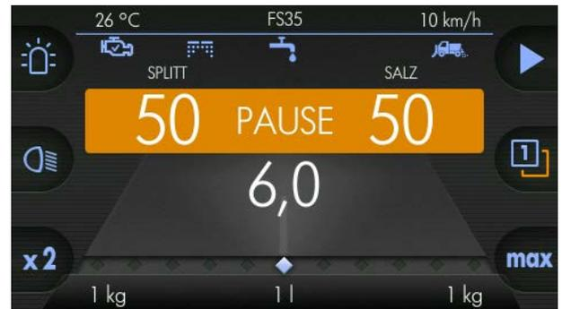
Turn right turning knob to change output rate of right chamber (Example: 57 g/m<sup>2</sup>) ⇒
