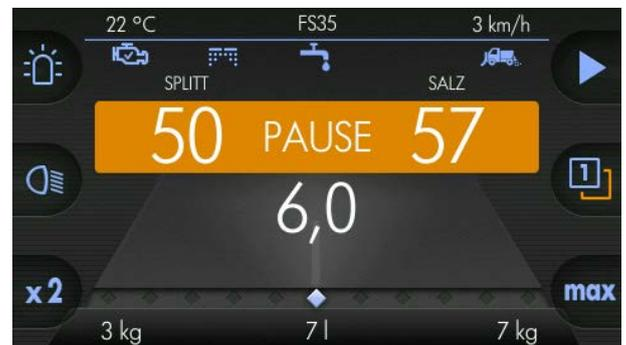
Turn left turning knob to change output rate of left chamber (Example: 58 g/m<sup>2</sup>) ⇒
