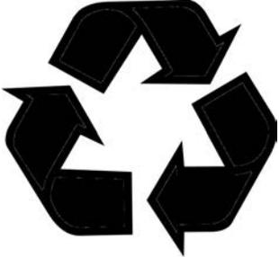
A black recycling symbol consisting of three arrows forming a triangle, representing a connection for recycled water.                                                                                                                                                             | Raccordo dell'acqua di riciclaggio                                           |
