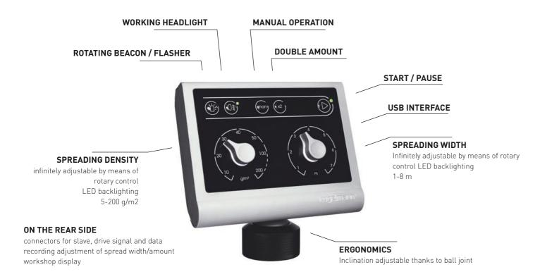
With the K-BASIC 2, kugelmann has managed to develop a control system reduced to the most essential. As an interface between operator and machine, the control system combines intuitive operation and precise spreading technology. Despite the high tech solution with intelligent feedback and control function, the K BASIC2 is easily understandable and its use quickly becomes routine. You have everything under control without compromising on your work.
