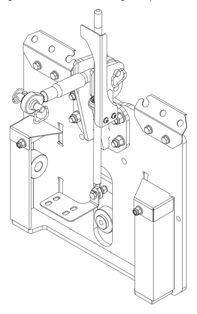
When the roller guide option is installed, adjust the snowplough's work position using the lifting device of the wheel loader.
