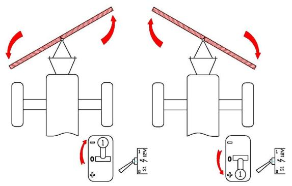
Switchover valve at 1: The right main blade swivels to the stop; the left main blade follows in the opposite direction.
