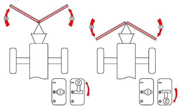
Functional drawing for variable snowplough on carrier vehicle with one double-acting controller and one electric switchover valve:
