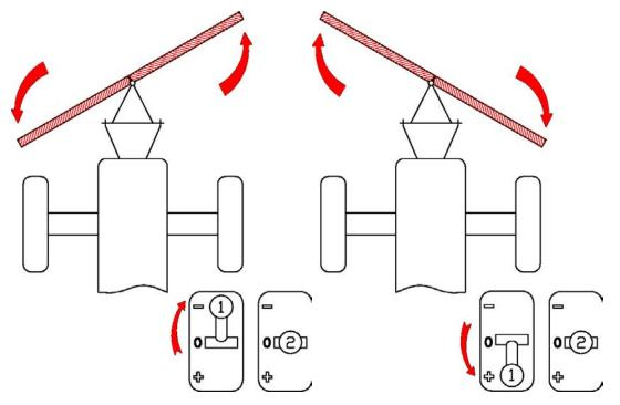
Controller 2: The right main blade swivels to the stop; the left main blade follows in the opposite direction.
