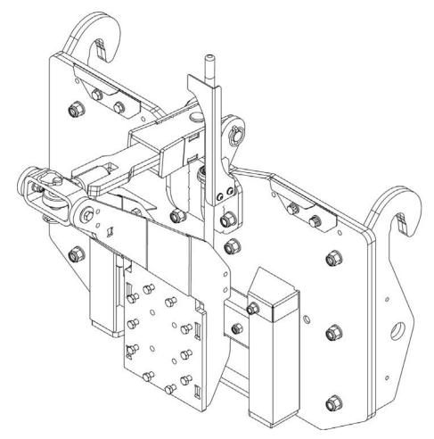
When the roller guide option is installed, adjust the snowplough's work position using the lifting device of the wheel loader.
